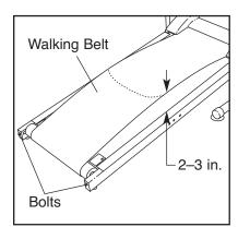
turn both rear roller adjustment bolts counterclockwise 1/4 of a turn. When the tension of the walking belt is correct, you should be able to lift each side of the walking belt 2 to 3 in. (5 to 7 cm). Walk on the treadmill for a few minutes. Repeat until the walking belt is properly tightened. Be careful to keep the walking belt centered.
